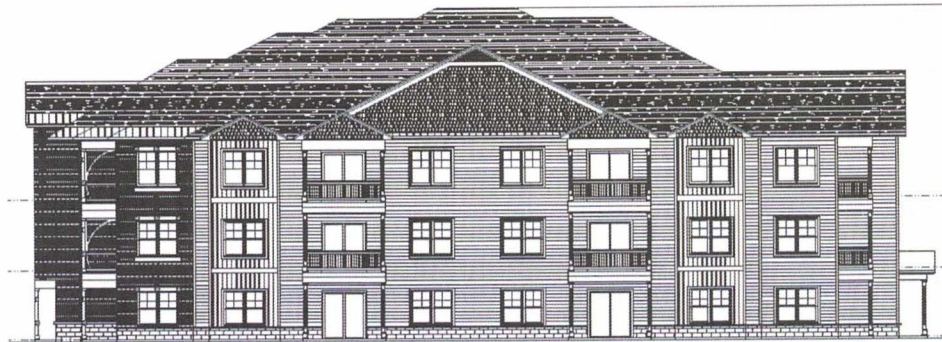
SOUTH ELEVATION - FACING SHARED ACCESS DRIVE 1/2" = 1'-0"
